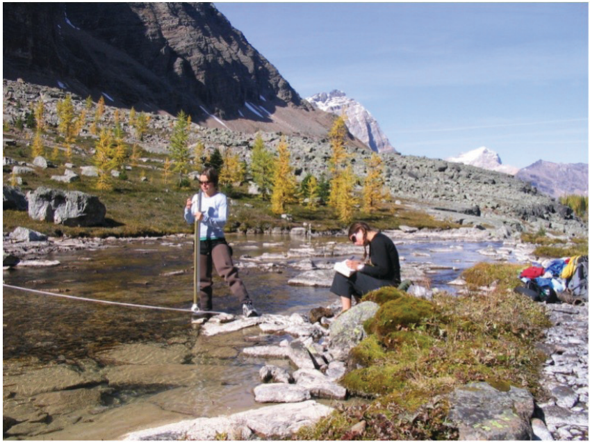
Students measuring groundwater outflow from a spring at the headwater of Opabin Creek in the Lake O'Hara watershed in Yoho National Park (September 17, 2008).
